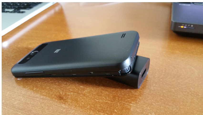
Figure 49 - Pry the back cover off of the phone.
