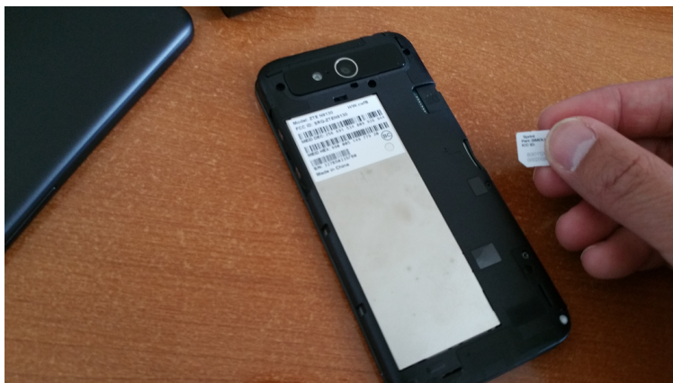
Figure 52 - Remove the card from its slot and replace the back cover.
