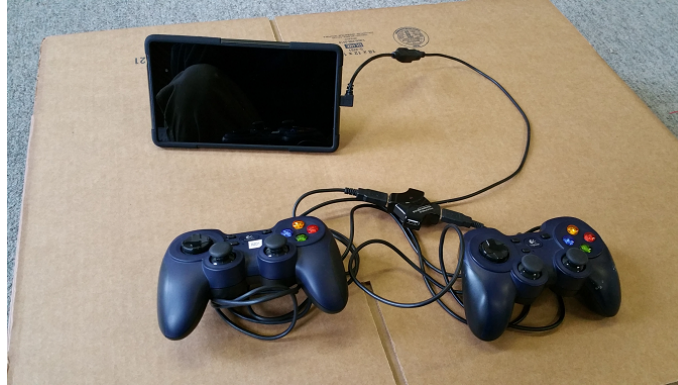
Figure 5 - Driver station hardware consists of a tablet, an adapter cable, a USB hub and two gamepads.
